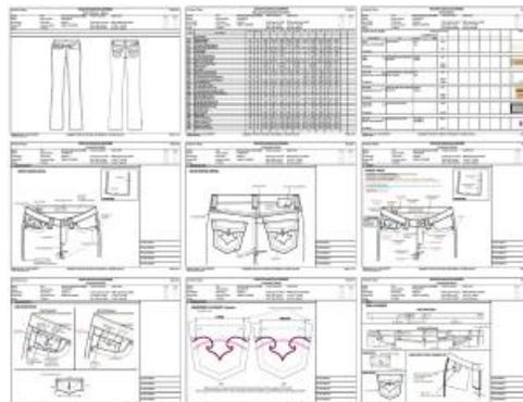
**Block** – A proven pattern that fits the target consumer, complete with the manufacturer’s characteristic style. It’s used to develop all subsequent styles. Has seam allowances.
